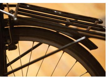
paired with the correct Kogswell fork, provides optimal handling for carrying a load on a rack above the front wheel.
